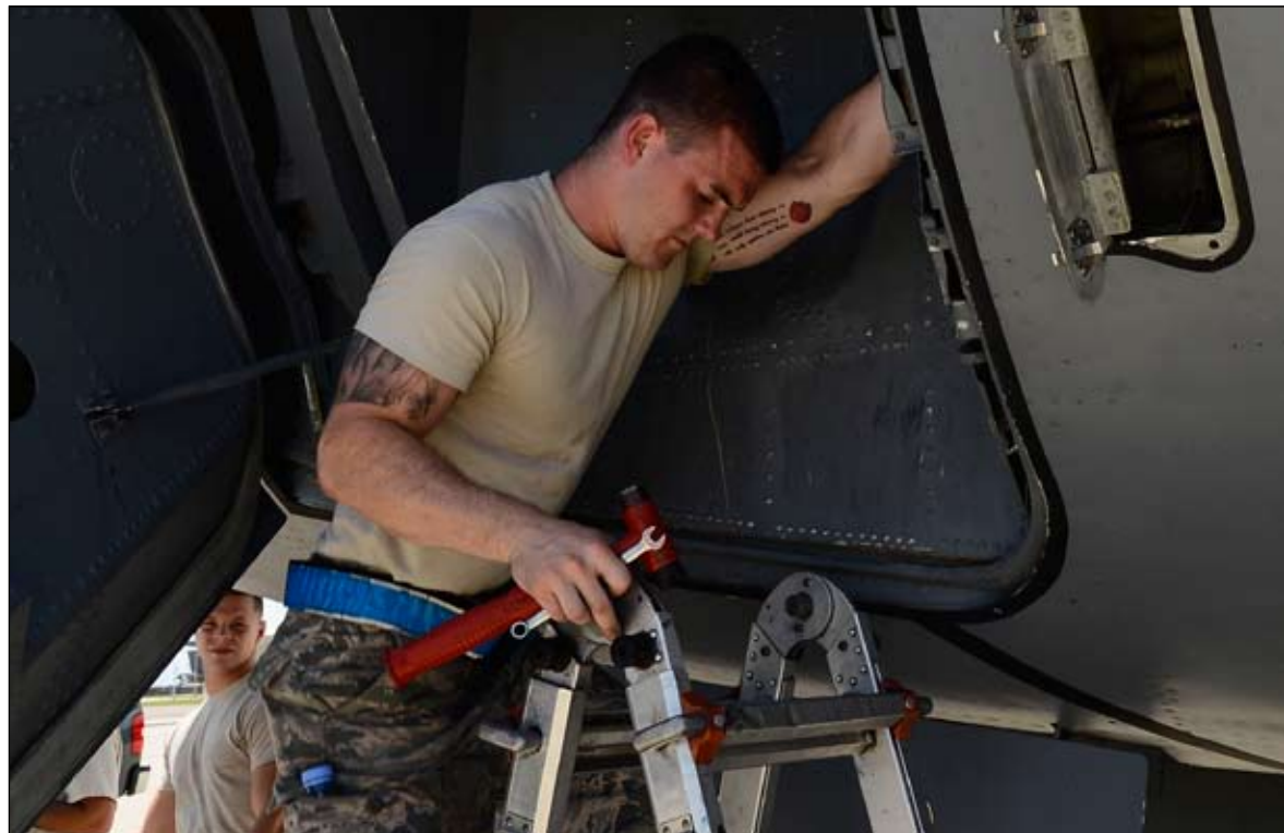
Senior Airman Stephen Rodgers, 6th Aircraft Maintenance Squadron crew chief, climbs the side of the nose well at MacDill Air Force Base, Aug. 12. Rodgers went inside the nose well to install the Improved Nose Wheel Snubber Brake.
