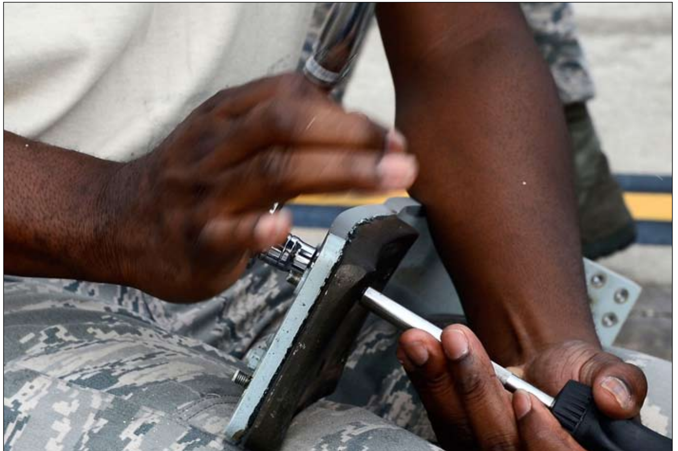
Airman 1st Class Cecil Sweeney, 6th Aircraft Maintenance Squadron crew chief, takes a brake liner off a snubber brake at MacDill Air Force Base, Aug. 12. The KC-135 Stratotanker uses the snubber brake to eliminate noise and vibration when the landing gear is retracted.
