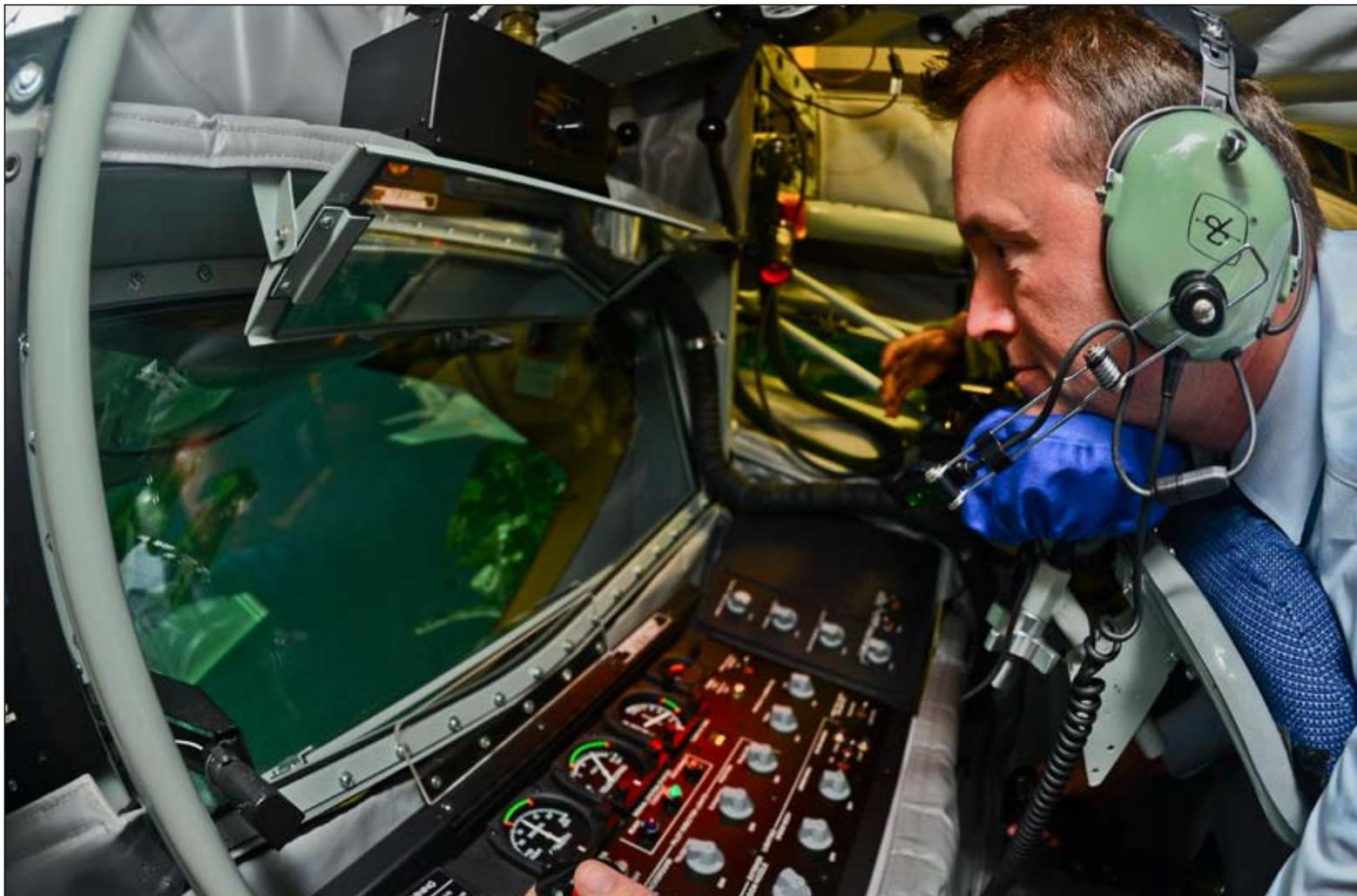
Acting Secretary of the Air Force Eric Fanning receives lessons on MacDill's Boom Operator Weapon Systems Trainer at MacDill Air Force Base, Aug. 29. The BOWST is a fully simulated, large-scale procedural trainer for aerial refueling with replicated aircraft systems, controls, and functions within a complete aircrew boom compartment.
