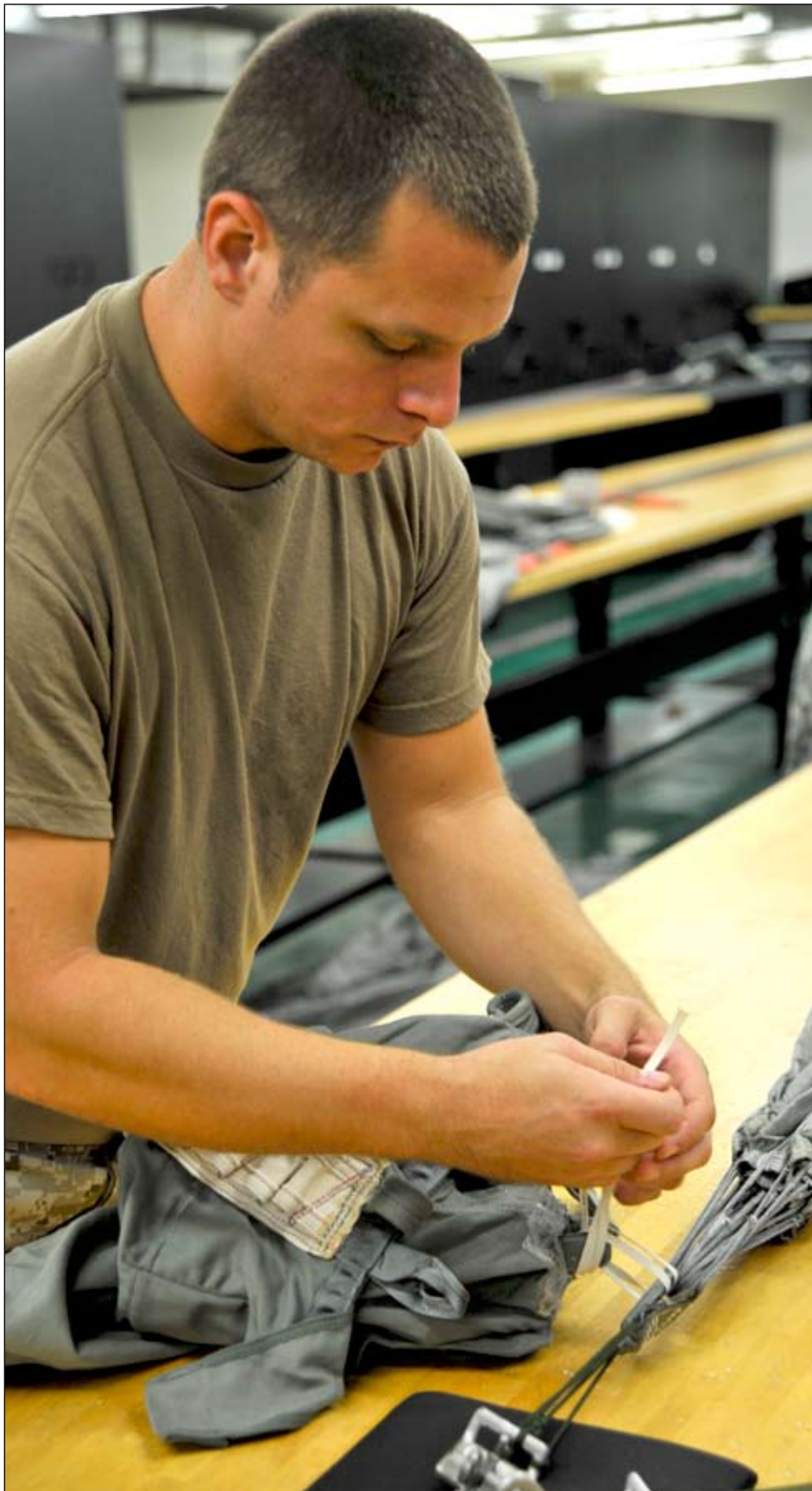
Petty Officer 2nd Class Joshua Goldsmith, United States Special Operations Command Central parachute rigger, secures a deployment bag to a canopy during parachute packing at MacDill, Sept. 18. Parachute connections are made using quarter-inch cotton webbing and are secured by tying a surgeon's knot.
