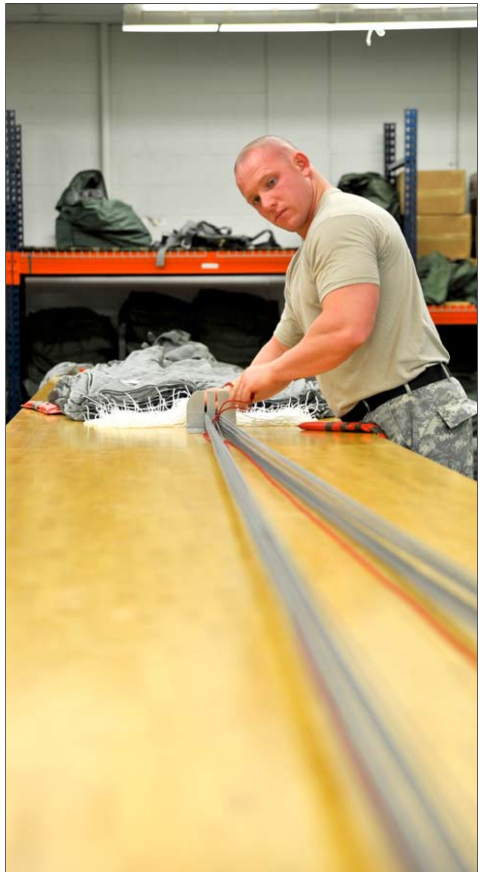
U.S. Army Sgt. Luke Allen, Joint Communications Support Element parachute rigger, adjusts a parachute's suspension lines during a parachute packing at MacDill Air Force Base, Sept. 18. The line continuity check is performed every time a parachute is packed to ensure no lines are crossed.
