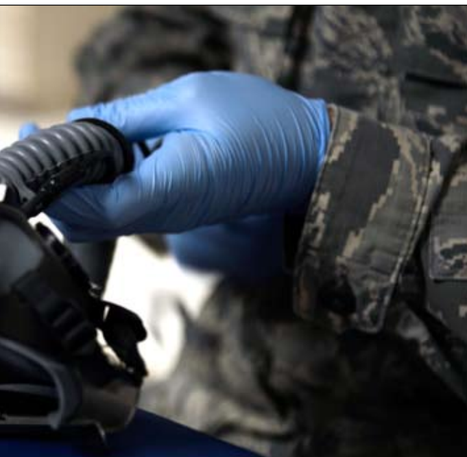
Senior Airman Taylor Clouse, 927th Operation Support Squadron aircrew flight equipment journeyman, performs routine maintenance on a MBU-12/P face mask at MacDill Air Force Base, Sept. 24. The HGU-55/P helmets and MBU-12/P face masks are inspected every 90 days.
