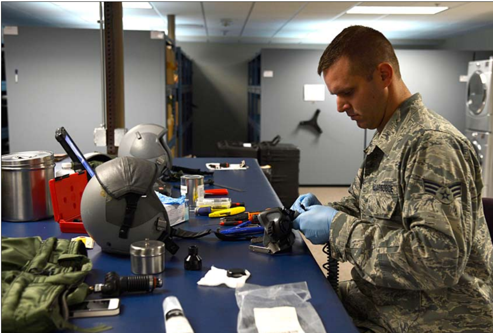
Senior Airman Taylor Clouse, 927th Operation Support Squadron aircrew flight equipment journeyman, performs routine maintenance on a MBU-12/P face mask at MacDill Air Force Base, Sept. 24. The HGU-55/P helmets and MBU-12/P face masks are inspected every 90 days.
