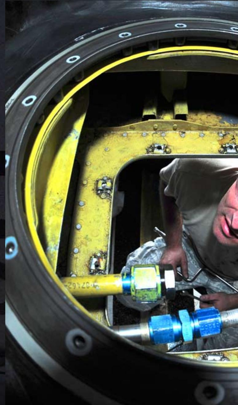
Senior Airman Bryan King, a 6th Maintenance Squadron aircraft fuels system craftsman, is working on a fuel bladder cell tank interconnect in the fuel bladder cell of a KC-135 Stratotanker, Oct. 10. King has been working a rigorous 24-hour schedule to identify
